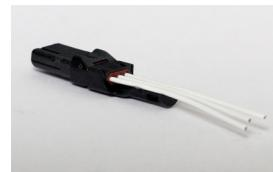
**STEP 1:** Using plastic extraction tool with proper color code corresponding to contact size, place wire in tool.
