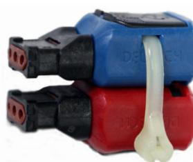
**OPTION 1:** Can mount connectors using cable tie <.10" (2.5mm) width x .04" (1.05) thick through the connector cable tie slot.
