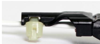
**STEP 1:** Backshell clips to the rear of the connector, fitting from either the top or the underside of the connector. Slide into position ensuring the side clips have latched into position.
