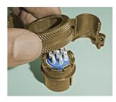
**STEP 5:** For barrels, add coupling nut to barrel and slide rear accessories on to cable.
