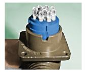
**STEP 3:** Insert insulator assembly into shell or barrel, aligning the key and keyway until rear of the insert is positioned just below the retaining spring ring ridge.
