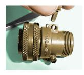
**STEP 7:** Thread endbell onto barrel/ shell. Slide cable clamp down the cable and thread onto the endbell. Tighten endbell and cable clamp using endbell accessory tools
