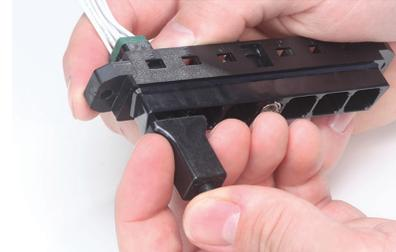
**STEP 2:** After crimping, wire should be visible through wire inspection hole.
