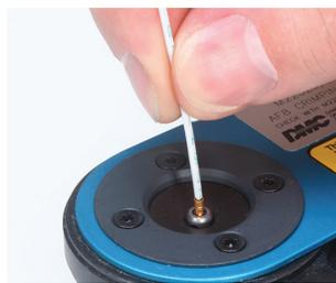
**STEP 1:** Fully insert wire into contact crimp pocket. Wire must be visible through wire inspection hole.
