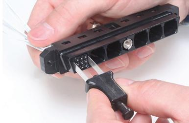
**STEP 1:** Insert contact into tool (use proper crimping tool as listed on preceding page). Crimp contact to wire. Tool will not open if contact is not fully crimped.
