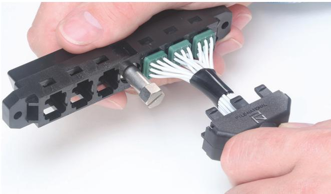
**STEP 1:** Tape wire bundle in area of cable clamp, and build up diameter to approx. 3/8 inches, if required. Align self-locking tines of the strain relief housing with the cavities adjacent to each module. Push the strain relief housing into place until the self-locking tines snap and lock strain relief into position. Assemble opposite half of strain relief housing to connector and tighten tie-strap to provide clamping force on the wire bundle.
