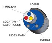
**STEP 3:** Select the proper locator position for your contact by rotating the locator until the proper color is aligned with the index mark. Push locator back down until it snaps into position
