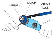
STEP 2: Open the AF8 (M22520/1-01) crimp tool by squeezing the handles. Push the latch on TH1A (M22520/1-02) to pop up the locator on the turret. Attach the turret to the AF8 crimp tool using the two captive hex bolts in the turret.
