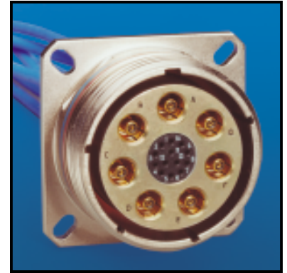
Special Hybrid Ground Plane Connector* with a standard MIL-DTL-38999 insert surrounded by a metal ground plane insert. This connector is designed for applications where the twinax contacts are required to be electrically bonded to a common ground while insulated M39029 signal or power contacts are also included for compact packaging.
