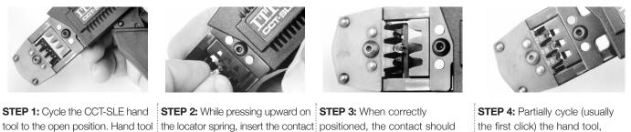
the first click) the hand tool, assuring that the upward-thrusting tails of the contact have started engaging with the top jaw of the tool. There is a slight tendency for the contact to roll out of vertical alignment.
