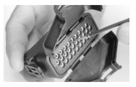
Insert contact from rear; an audible snap can be felt and heard. A slight pull in the opposite direction will confirm complete insertion.
