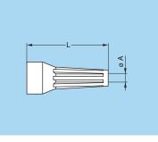
A bend relief made from thermoplastic polyurethane elastomer can be fitted over LEMO plugs and sockets that are supplied with nut for fitting such bend relief.
