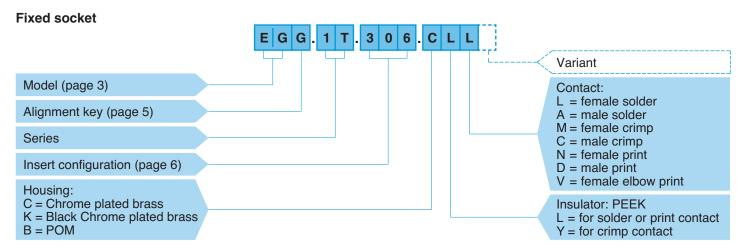
**EGG.1T.306.CLL** = fixed socket, nut fixing, with key (G), 1T series, multipole type with 6 contacts, outer shell in chrome-plated brass, PEEK insulator, female solder contacts.
