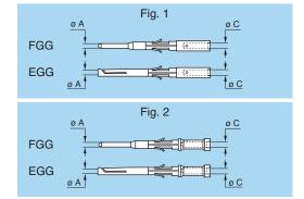
**Note:** a wide variation of strand number and diameter combinations are quoted as being AWG, some of which do not have a large enough cross section to guarantee a crimp as per either MIL-C-22520/1-01 or /7-01.
