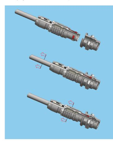
The LEMO self-latching system allows the connector to be mated by simply pushing the plug axially into the socket.
