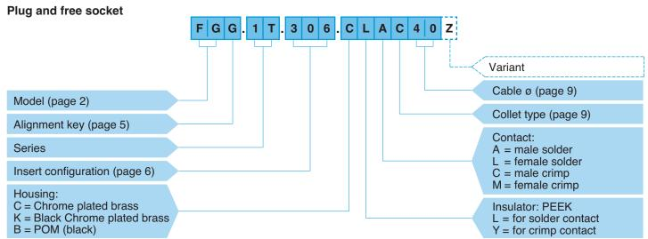
**FGG.1T.306.CLAC40Z** = Straight plug with key (G) and cable collet for bend relief, 1T series, multipole type with 6 contacts, outer shell in chrome-plated brass, PEEK insulator, male solder contacts, C type collet for 4.0 mm diameter cable and nut for fitting a bend relief.
