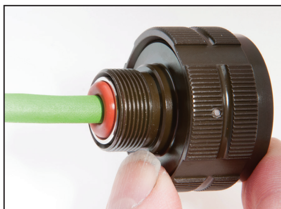
24. The plug is fully installed when the back of the seal carrier is flush with the connector as shown
