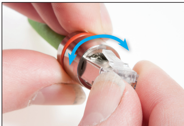
21. Rotate the seal carrier against the plug to confirm alignment
