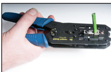
18. Insert plug and cable into crimp tool and fully close tool
