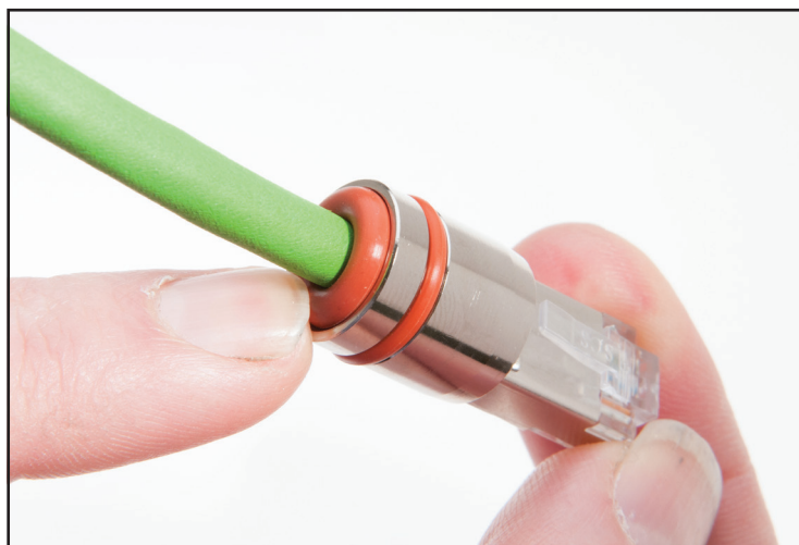
22. Push O-ring against the seal carrier to hold in place
