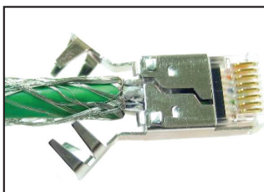
15. Gently insert assembly into housing
