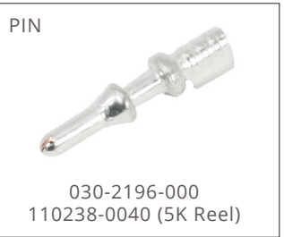
Insulation Support: Crimps contact to wire and insulation Strip Length Inches (mm): .185 - .185 (3.94 - 4.70mm)
