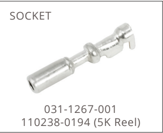
Non-Insulation Support: Crimps contact to wire only Strip Length Inches (mm): .185 - .220 (4.70 - 5.59mm)
