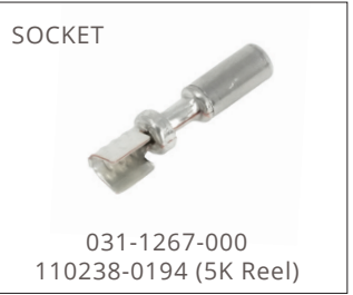
Non-Insulation Support: Crimps contact to wire only Strip Length Inches (mm): .185 - .220 (4.70 - 5.59mm)
