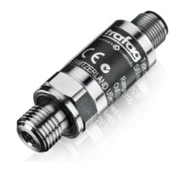
The switching outputs include the functions hysteresis and window with the option normally open and normally closed. A delay time is provided for each switching output. For the 2nd switching output is a monitoring mode "Device Ready" available. In this mode the output changes the state if the device has successfully completed the start-up phase. In case of an error during operation the status will change back to the normal state.
