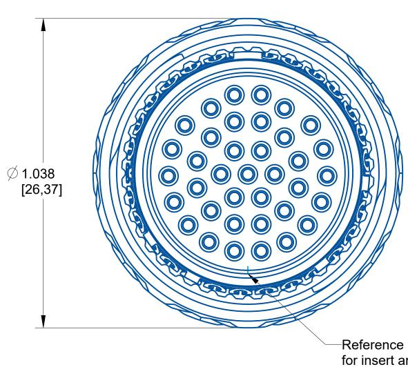
Reference MIL-STD-1560C for insert arrangement details. For non-MS arrangements consult Amphenol.
